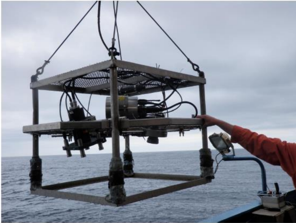
Figure 4. Drop camera frame with video and still imaging system.
