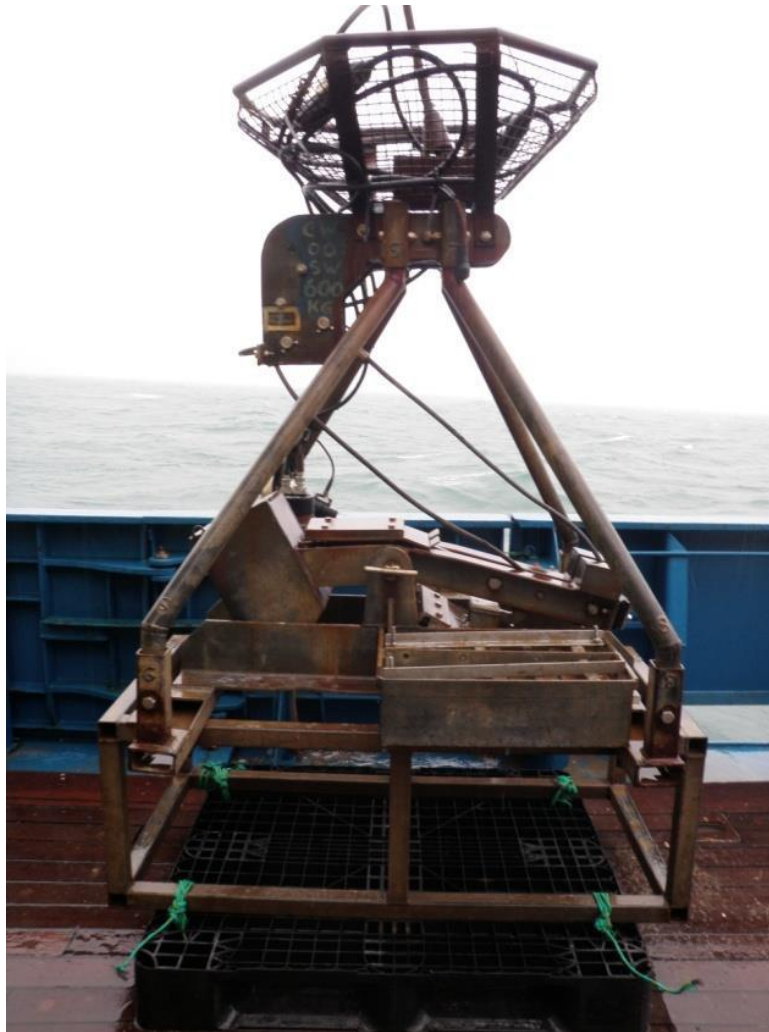
Figure 3. Mini Hamon grab with video camera (HamCam).
