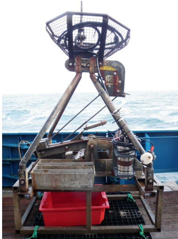
Figure 7. Mini Hamon grab with video camera (HamCam).
