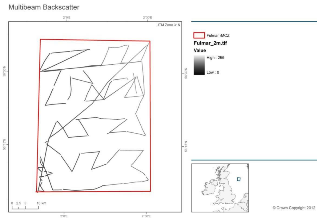
Figure 4. Backscatter from opportunistic multibeam lines collected on transit between ground truth stations.
