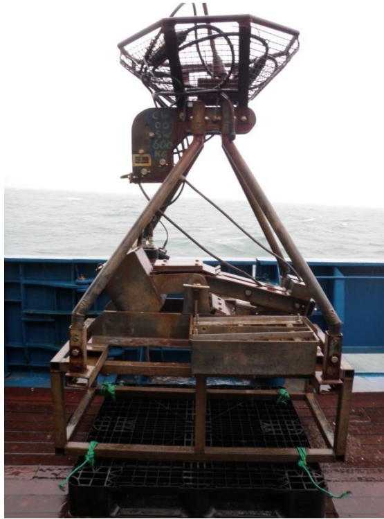
Figure 2. Mini Hamon grab with video camera (HamCam).
