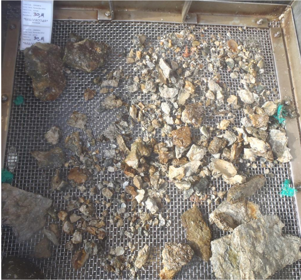
Figure 7. Sediment retained on the 5mm screening mesh at station A27, with 'mudstone' present.
