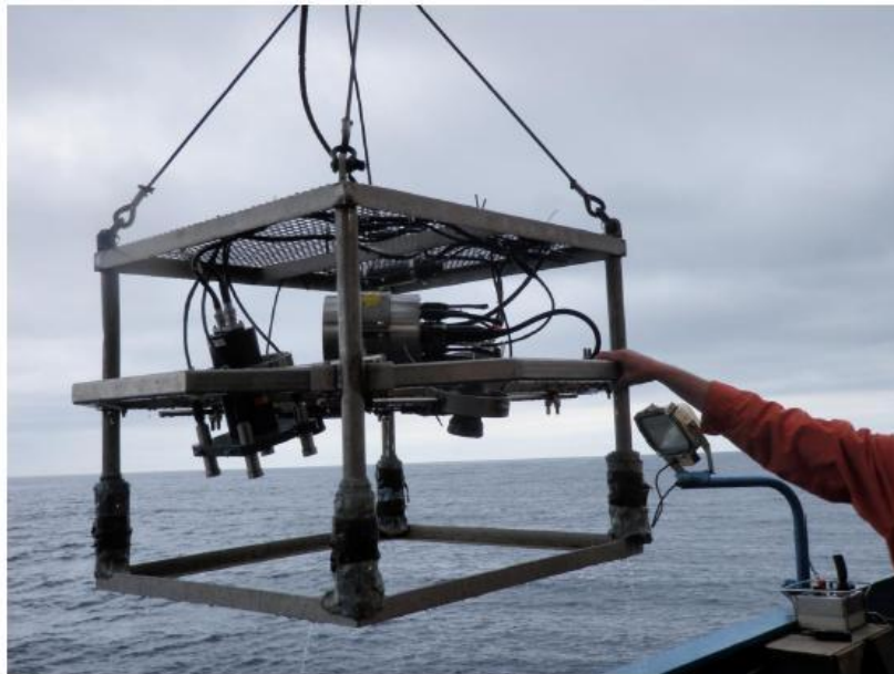
Figure 4. Drop camera frame with video and still imaging system and USBL beacon
