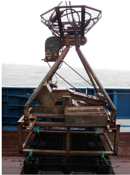
Figure 2. Mini Hamon grab with video camera (HamCam).
