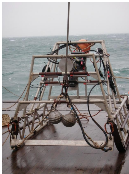
Figure 3. Camera sledge with video and still imaging system.
