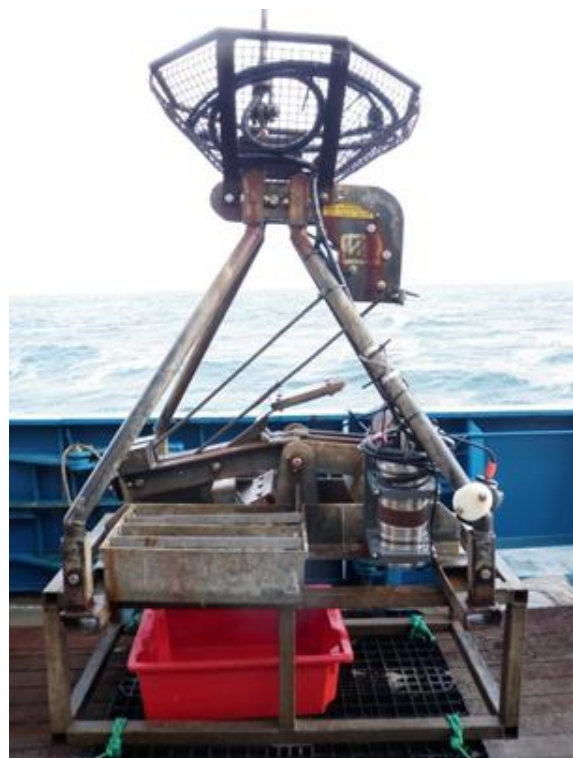
Figure 3. Mini Hamon grab with video camera (HamCam).
