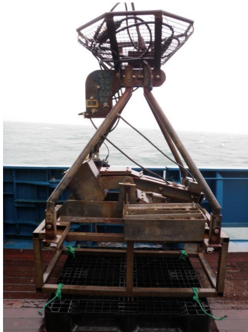
Figure 2. Mini Hamon grab with video camera (HamCam).
