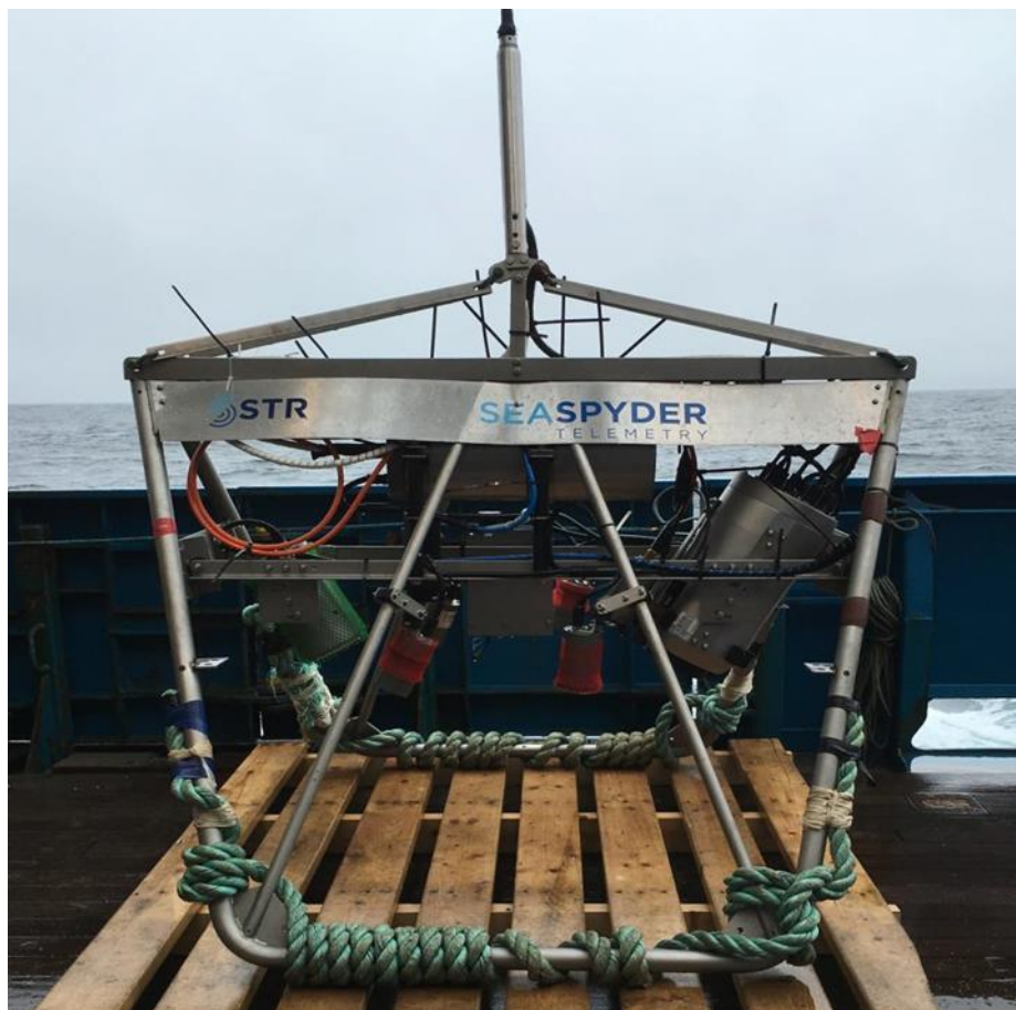
Figure 4. STR (Subsea Technology and Rentals) drop frame with video and still imaging system.
