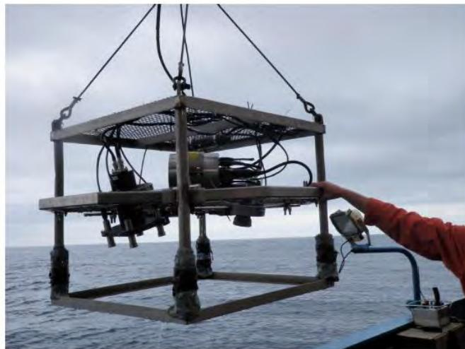
**Figure 8.** Drop-camera frame fitted with video and still imaging system, © Cefas 2012.
