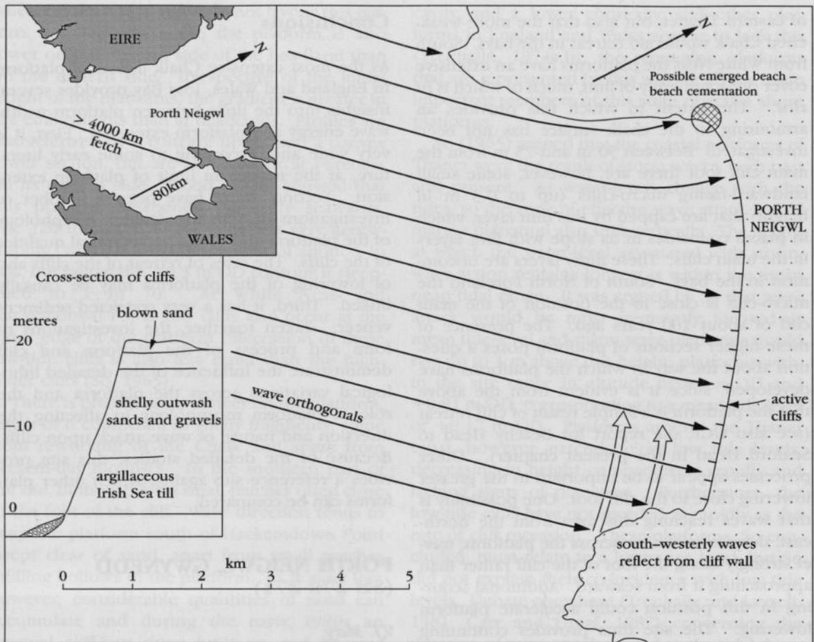
**Figure 4.39** Wave refraction and reflection in Porth Neigwl. Wave orthogonals show the direction of travel of waves and are drawn at right angles to the wave crest. Open arrows are also orthogonals for reflected waves.
