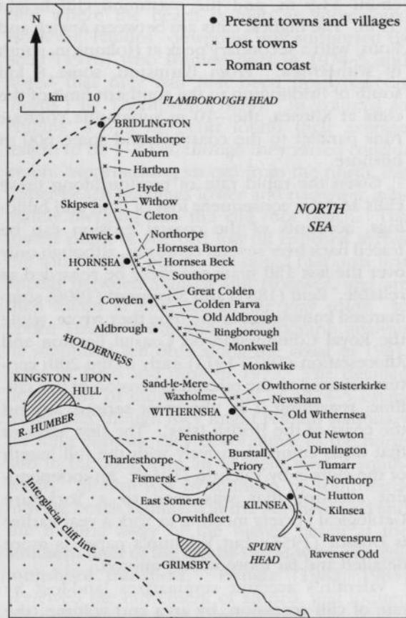
**Figure 4.40** Lost villages of the Holderness coast. As the till has been easily eroded for hundreds of years at rates of 2 m a<sup>-1</sup>, there has been substantial loss of agricultural land and villages. (After Hansom, 1988)
