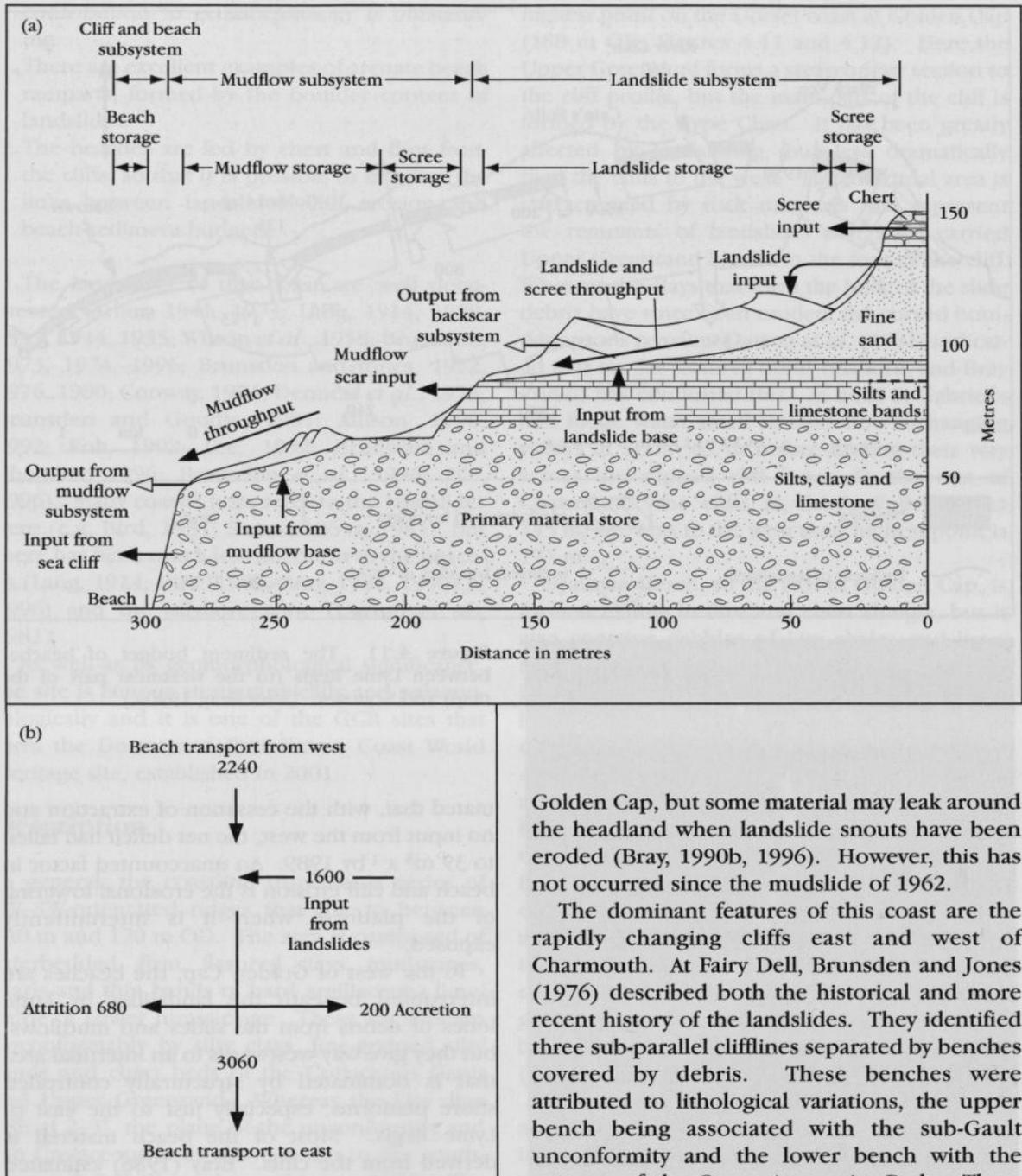
**Figure 4.13** (a) Cross-section of the Black Ven system (Lyme Regis to Golden Cap GCR site) and sediment supply to its beach. See also Figure 4.11. In (b) the volumes of sediment (in  $\text{m}^3 \text{a}^{-1}$ ) moving through the Black Ven beach are given. (Based on Brunsden, 1973 and Bray, 1990a.)
