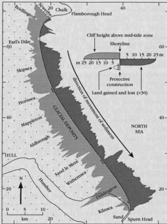
**Figure 4.41** The relationship between cliff height and erosion along the Holderness coast. (After Valentin, 1971, in Steers, 1971a). For the cliff height profile, the vertical exaggeration is  $\times 30$ .
