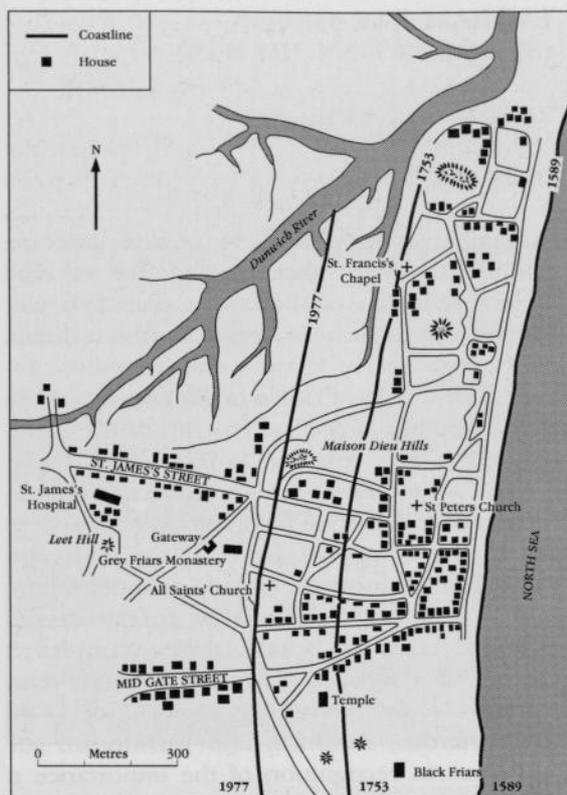
**Figure 4.3** Retreat of the coastal cliff at Dunwich, Suffolk, plotted on the 1589 map of Agas; the 1977 cliff top as surveyed by A.H.W Robinson. (After Robinson, 1980a, p.141)
