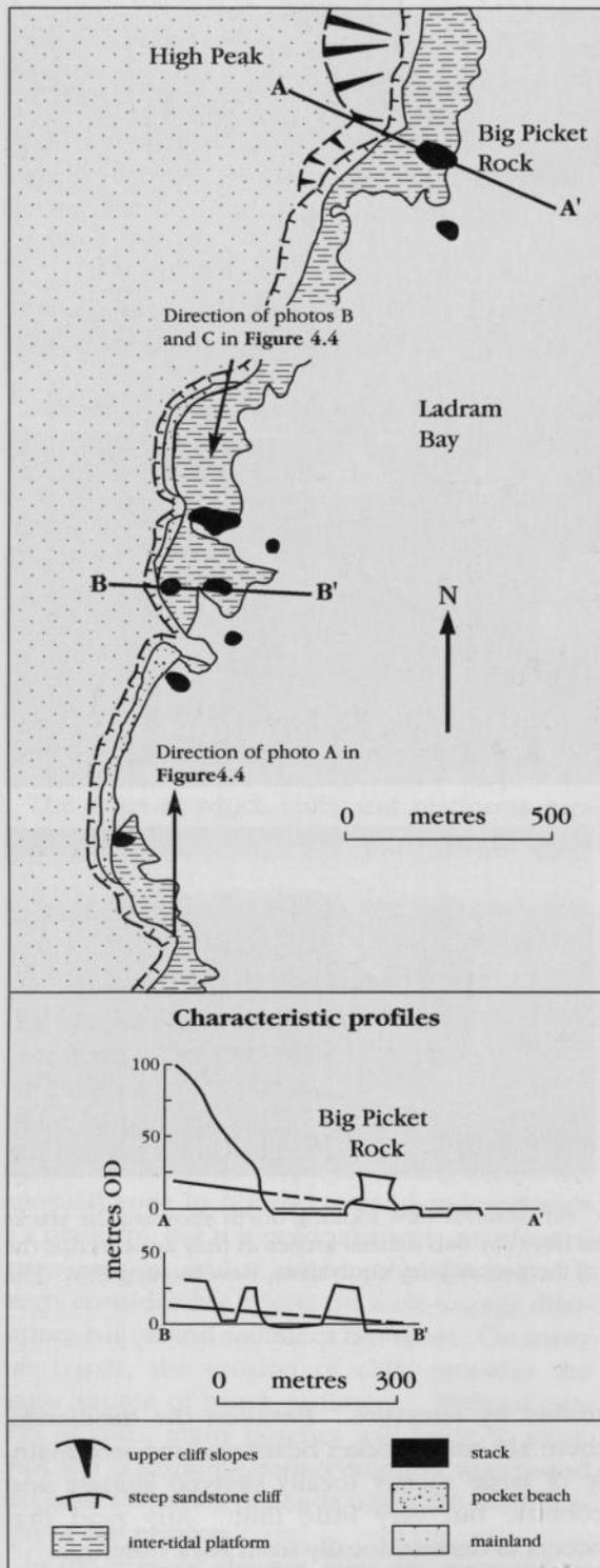
**Figure 4.5** The cliffline, platforms and stacks at Ladram Bay. Characteristic profiles are shown (A-A' and B-B'). Of particular note are the absence of stacks below the high cliffs, the presence of strata with fewer discontinuities in the lower stacks, and the tendency for stacks to be associated with headlands.
