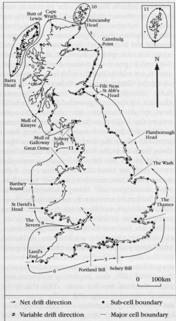
Figure 1.6 Littoral sediment cells and subcells and direction of littoral drift. After Motyka and Brampton, 1993 and HR Wallingford, 1997. Cells are numbered 1 to 7 anticlockwise from St. Abb's Head for Scotland and there are three subcells within the Orcadian cell; clockwise from St Abb's Head, cells are numbered 1–11 for England and Wales.
