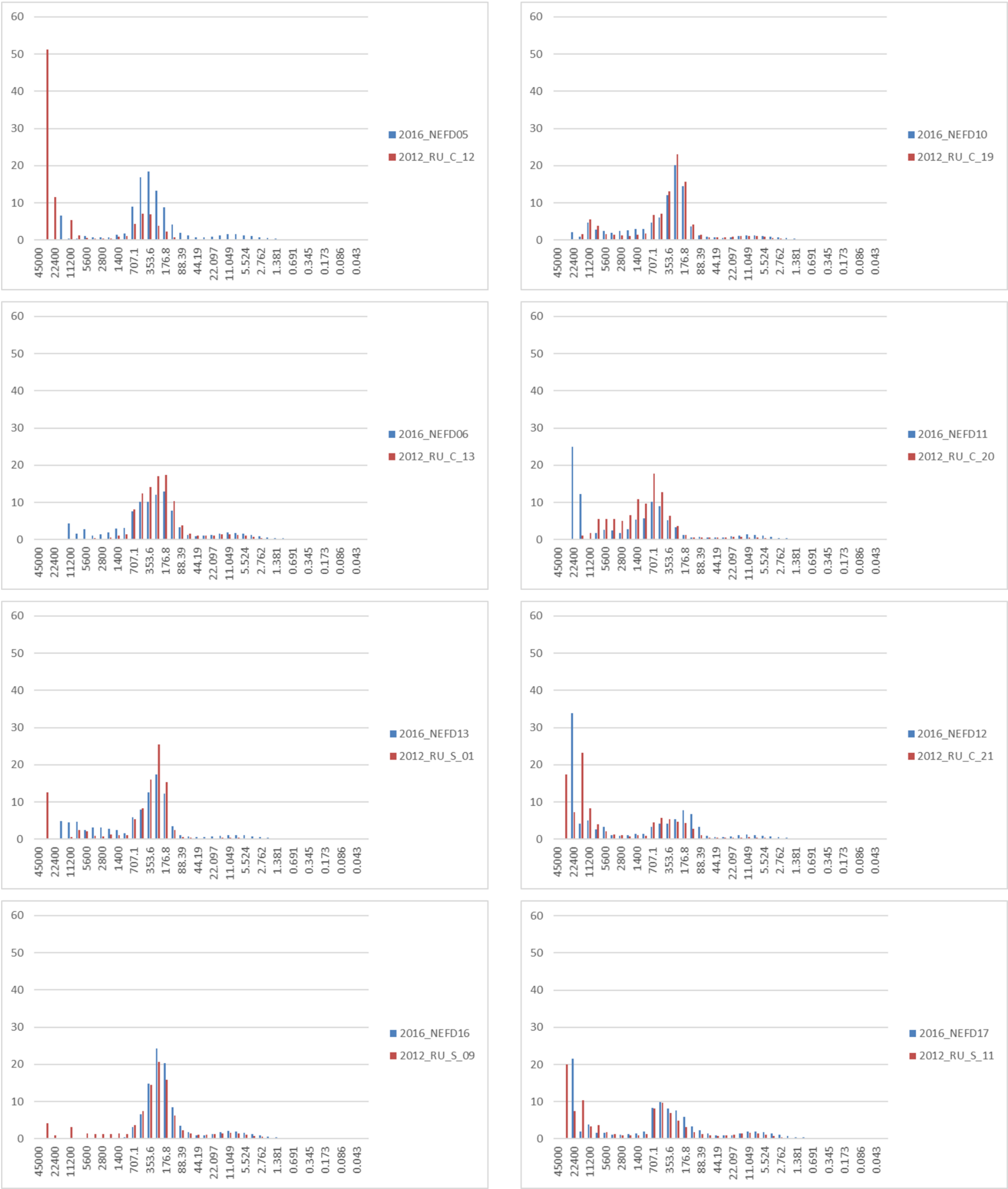
Figure 17. Frequency histograms (x axis = \mu\text{m} , y axis = %) showing the differences in particle size distribution across the ten stations at North East of Farnes Deep MCZ where different Entropy groups were assigned in 2012 (red) and 2016 (blue).
