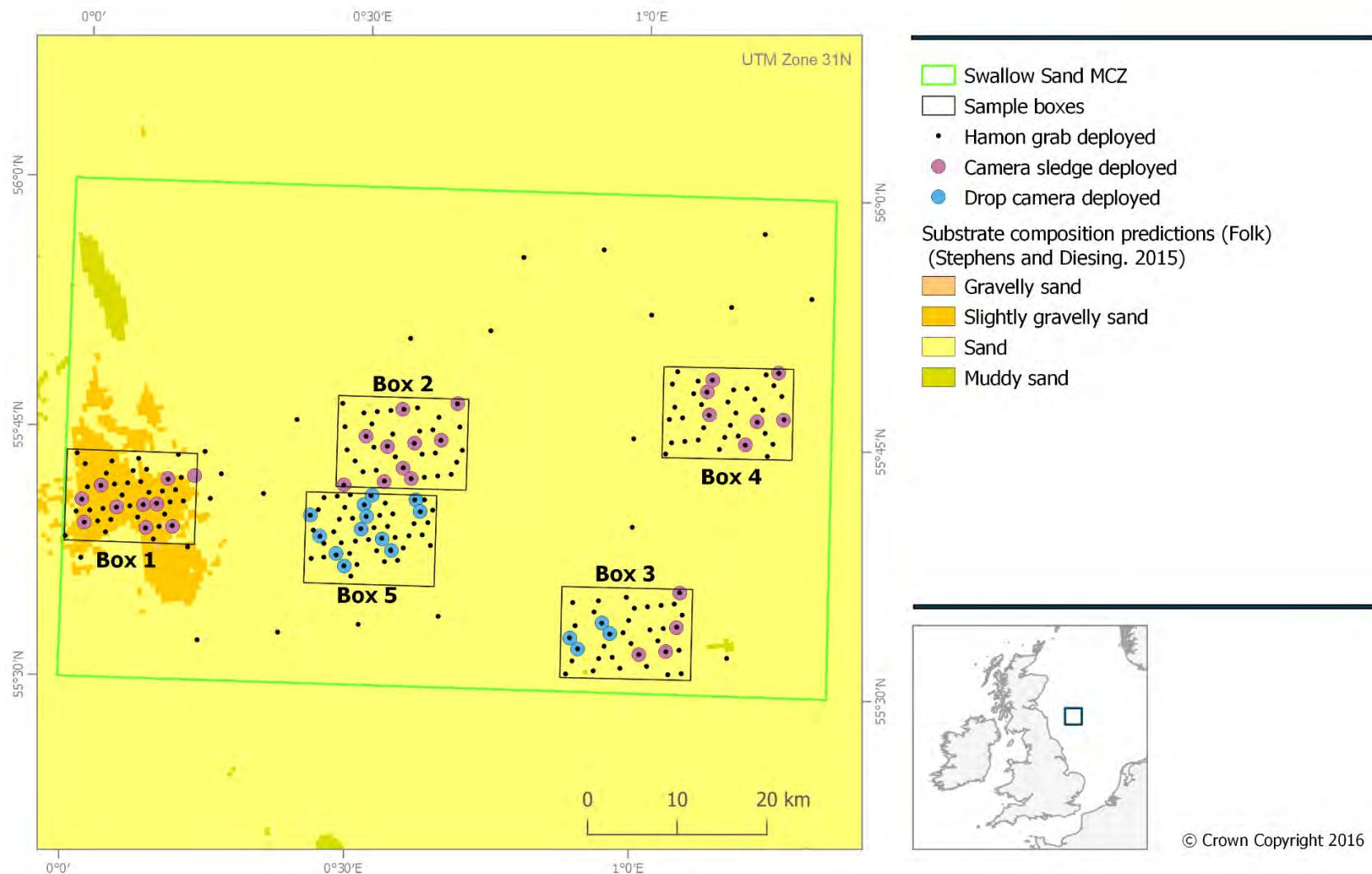
**Figure 12.** The five survey boxes and all sampling stations visited with the Hamon grab, camera sledge and drop camera at Swallow Sand MCZ. The base map shows predicted broad-scale habitats.
