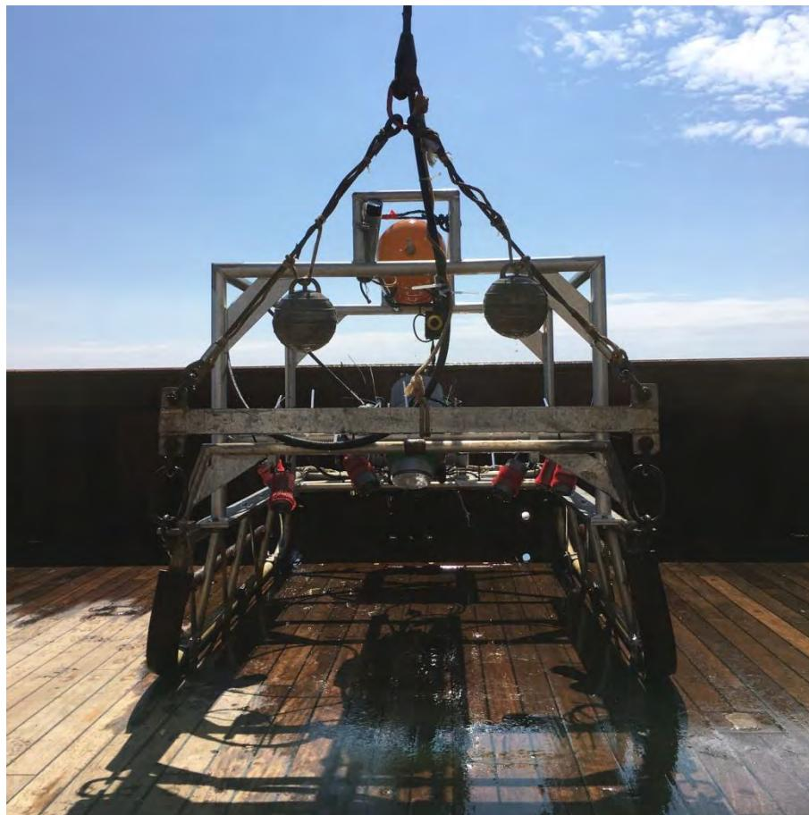
**Figure 8.** Camera sledge with video and still imaging system.
