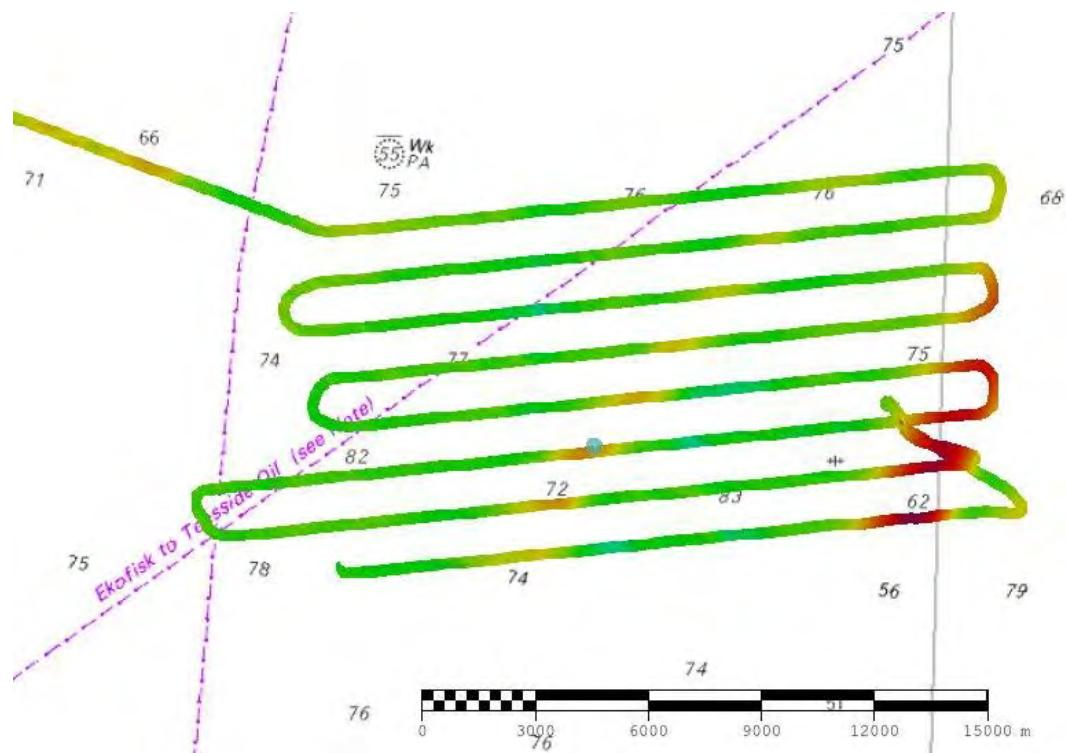
**Figure 11.** MBES bathymetric data collected over priority Box 3.
