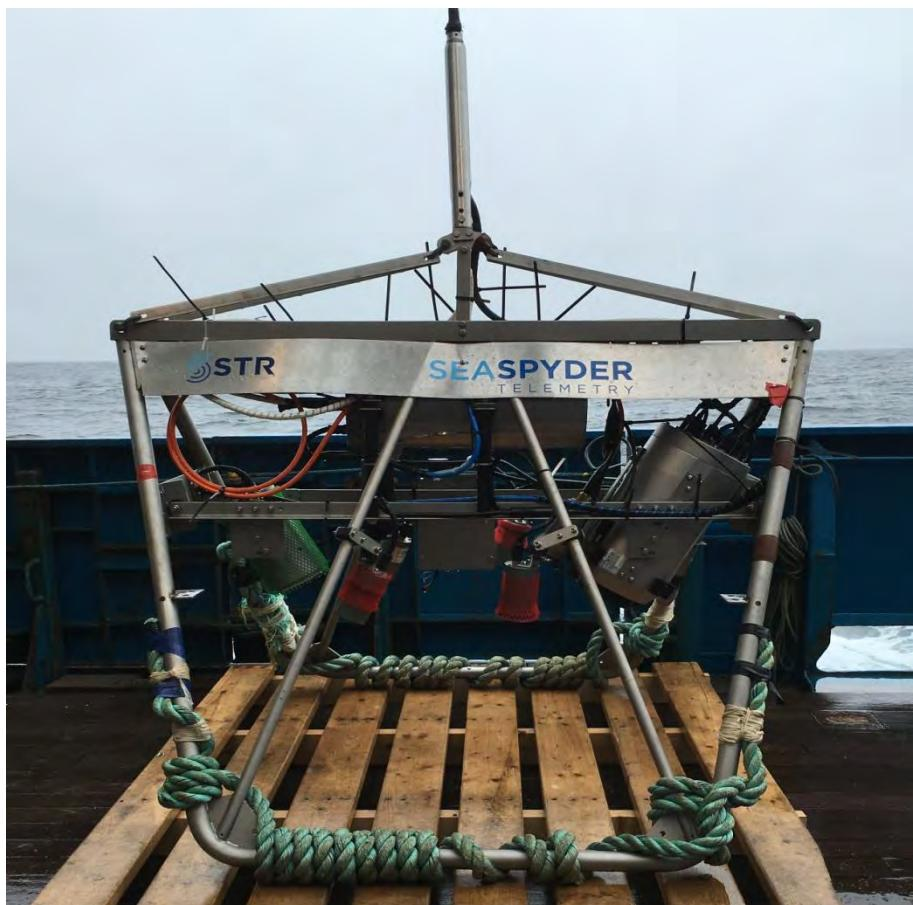
**Figure 9.** STR drop frame with video and still imaging system.
