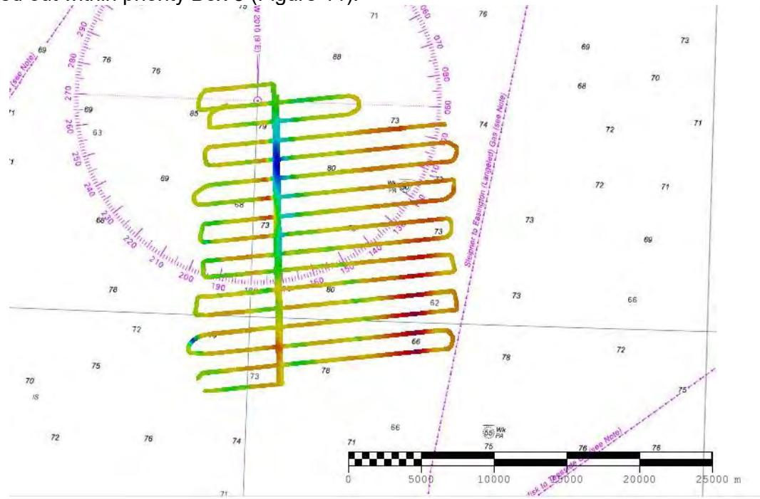
**Figure 10.** MBES bathymetric data collected over priority boxes 2 and 5.
