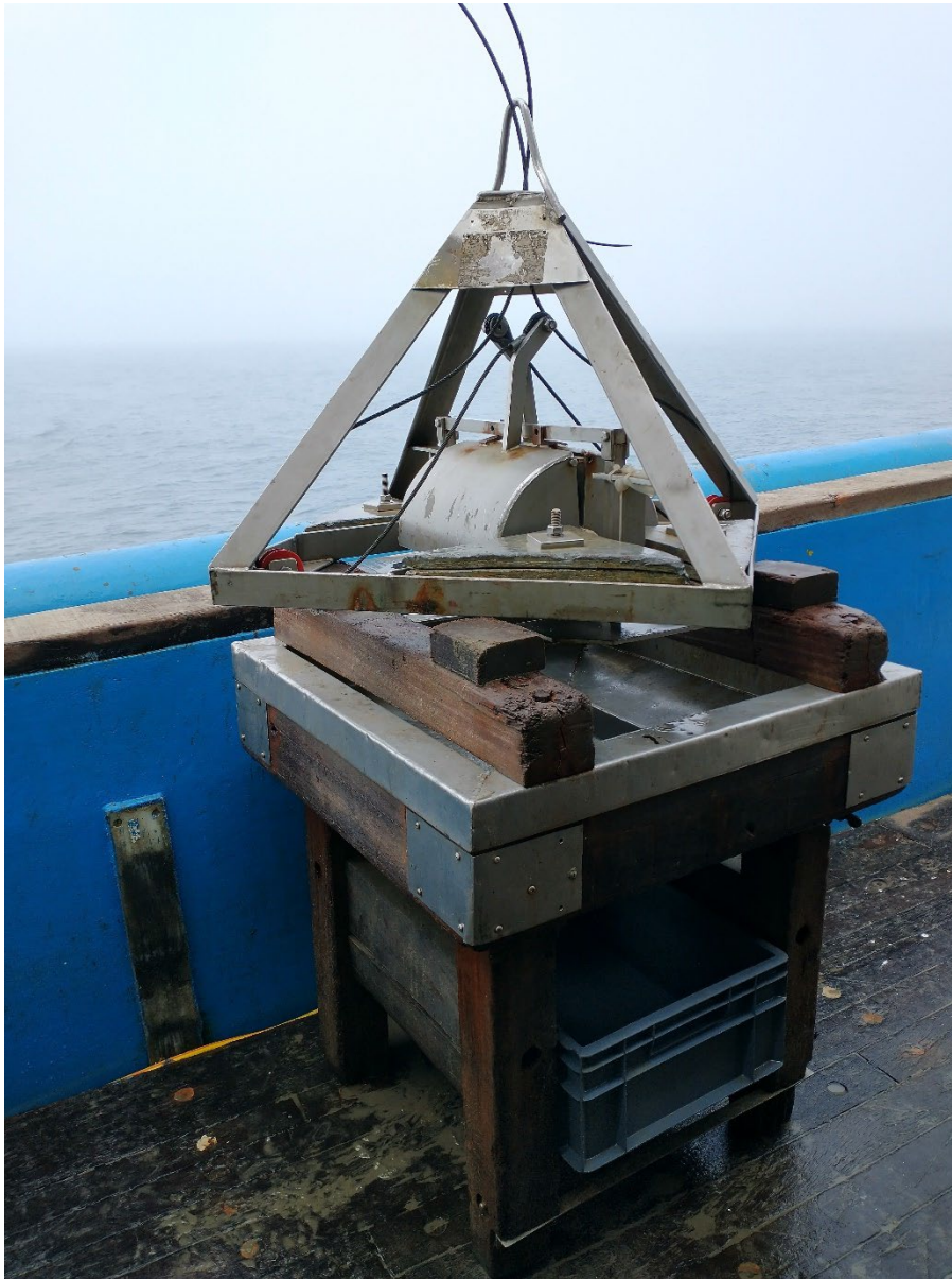
Figure 6. Photograph of the 0.1 m 2 Day grab used on the 0723S survey of Central Fladen Nature Conservation MPA.
