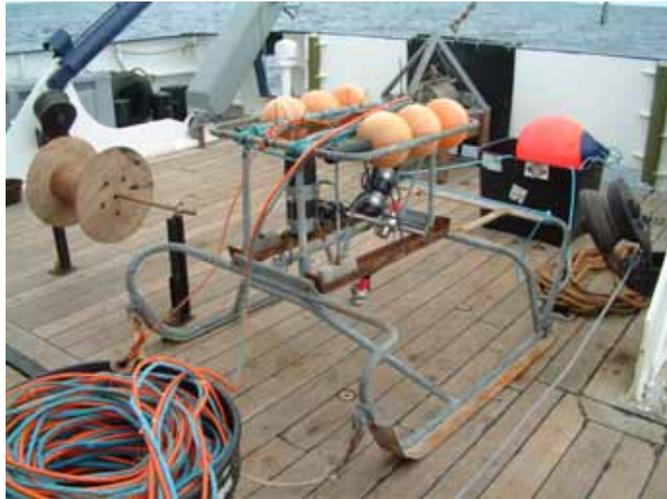
Figure 6.1.1: Camera sledge with Photosea still camera system (black housings), and Rovtech video camera and lights (red plug retainers). The umbilical cable is coiled in the tub on the left and the tail rope buoy is to the right.
