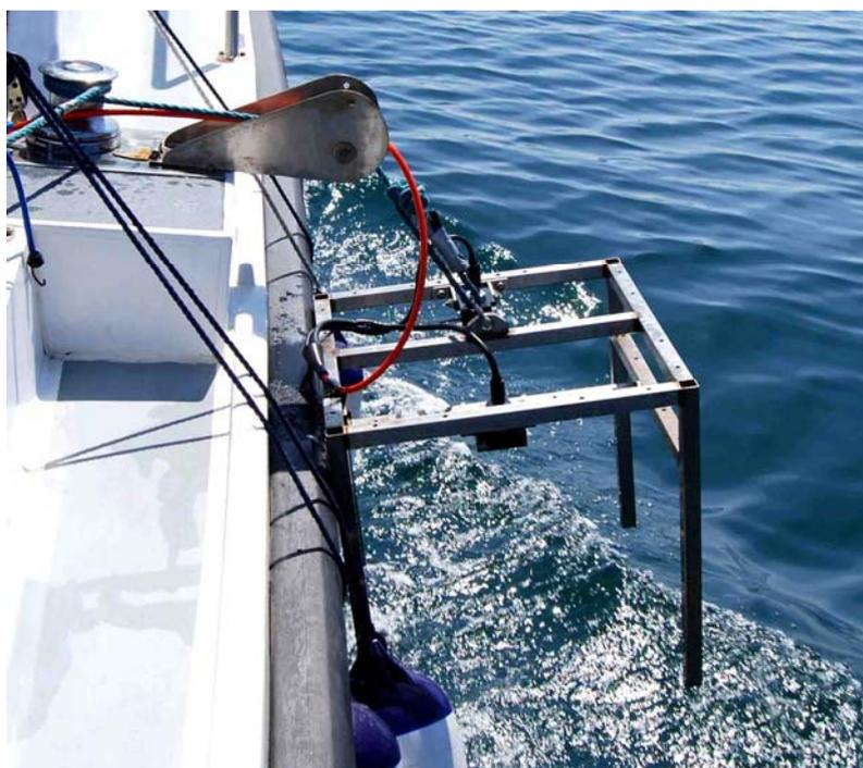
**Figure 3.5.** Drop camera, light and stainless steel frame ready for deployment to 20m depth off Rathlin Island, Northern Ireland.
