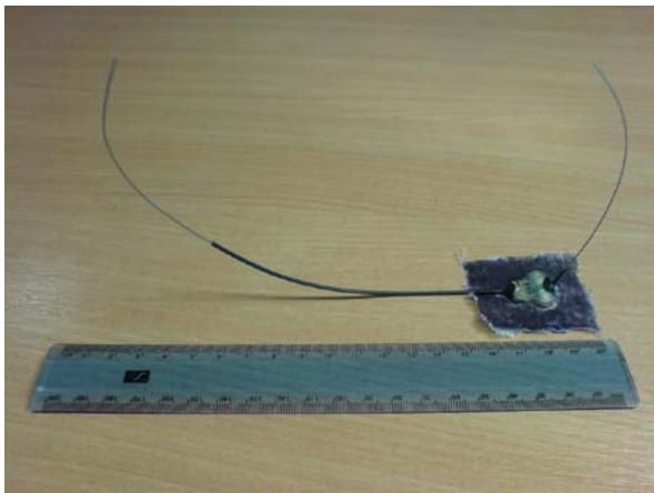
**Figure 7.** Radio tracking tag with antennae ready to attach to bird, with a ruler to show scale and size.
