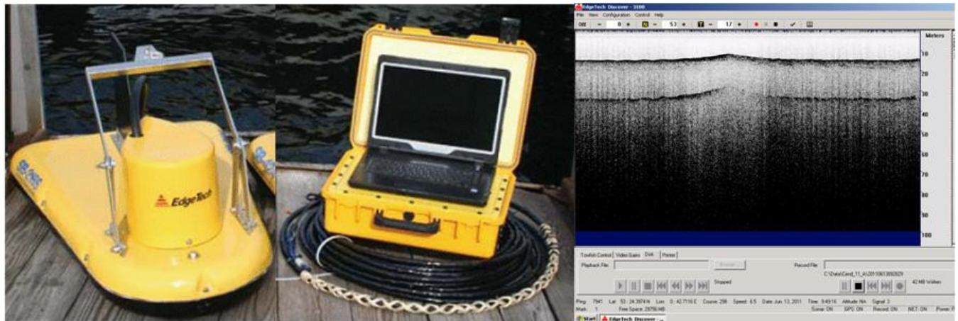
Figure 28. Portable sub-bottom profile system, top side processor and output
