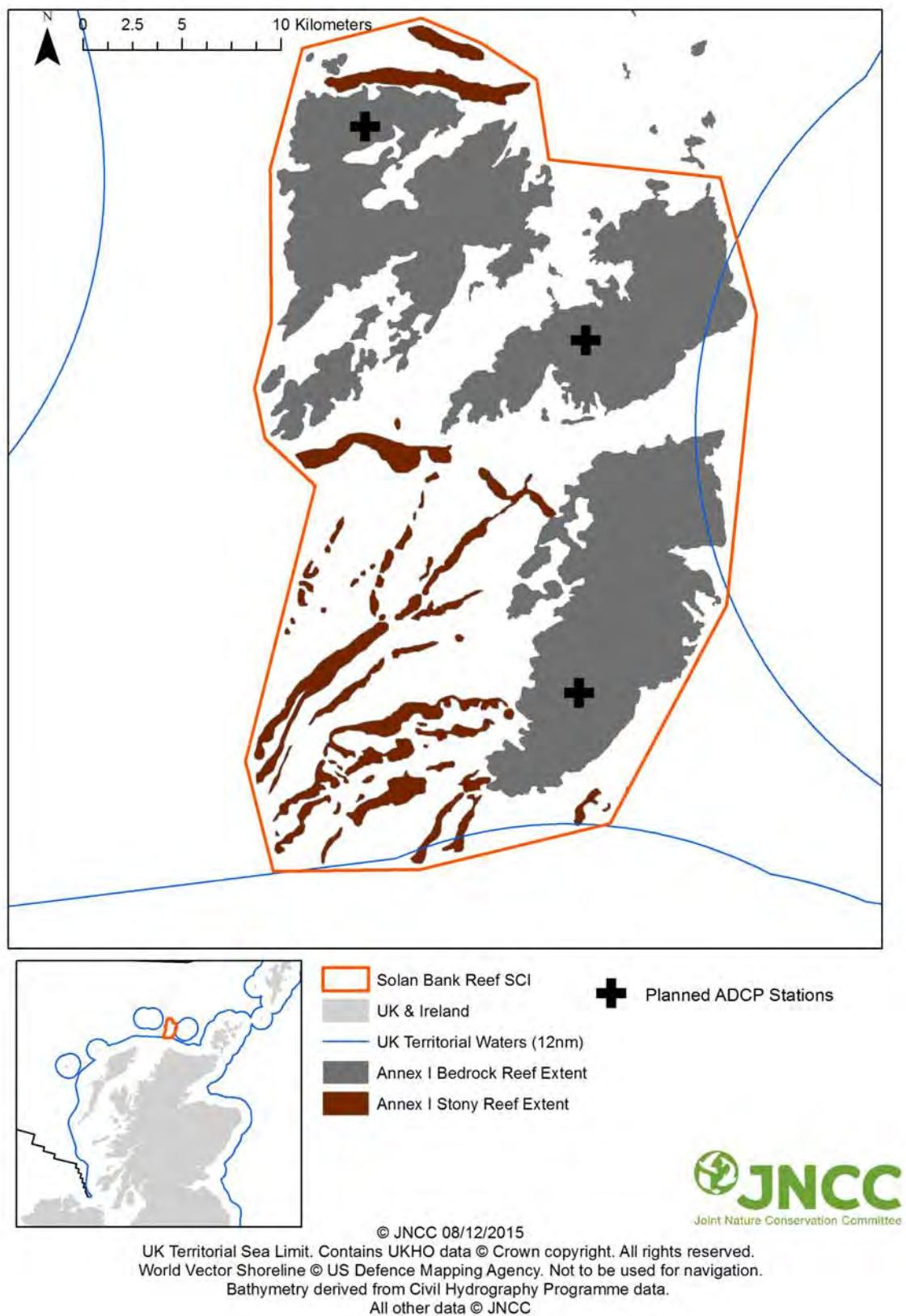
**Figure 5.** Contingency stations identified for ADCP deployment to measure bottom current flow rate and direction.
