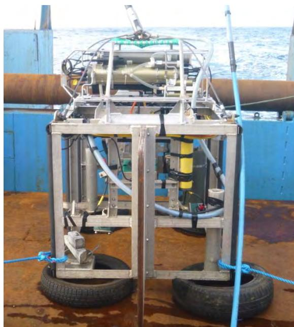
**Figure 6.** Drop Frame used on 1714S Solan Bank Reef SCI survey.
