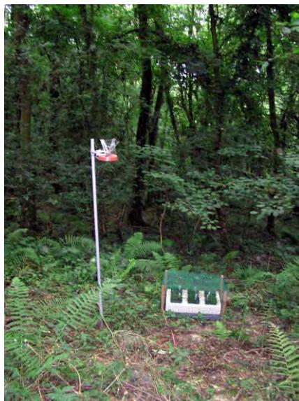
**Figure 2.3.** Ammonia monitoring at Piddles Wood 40 m from the poultry unit.
