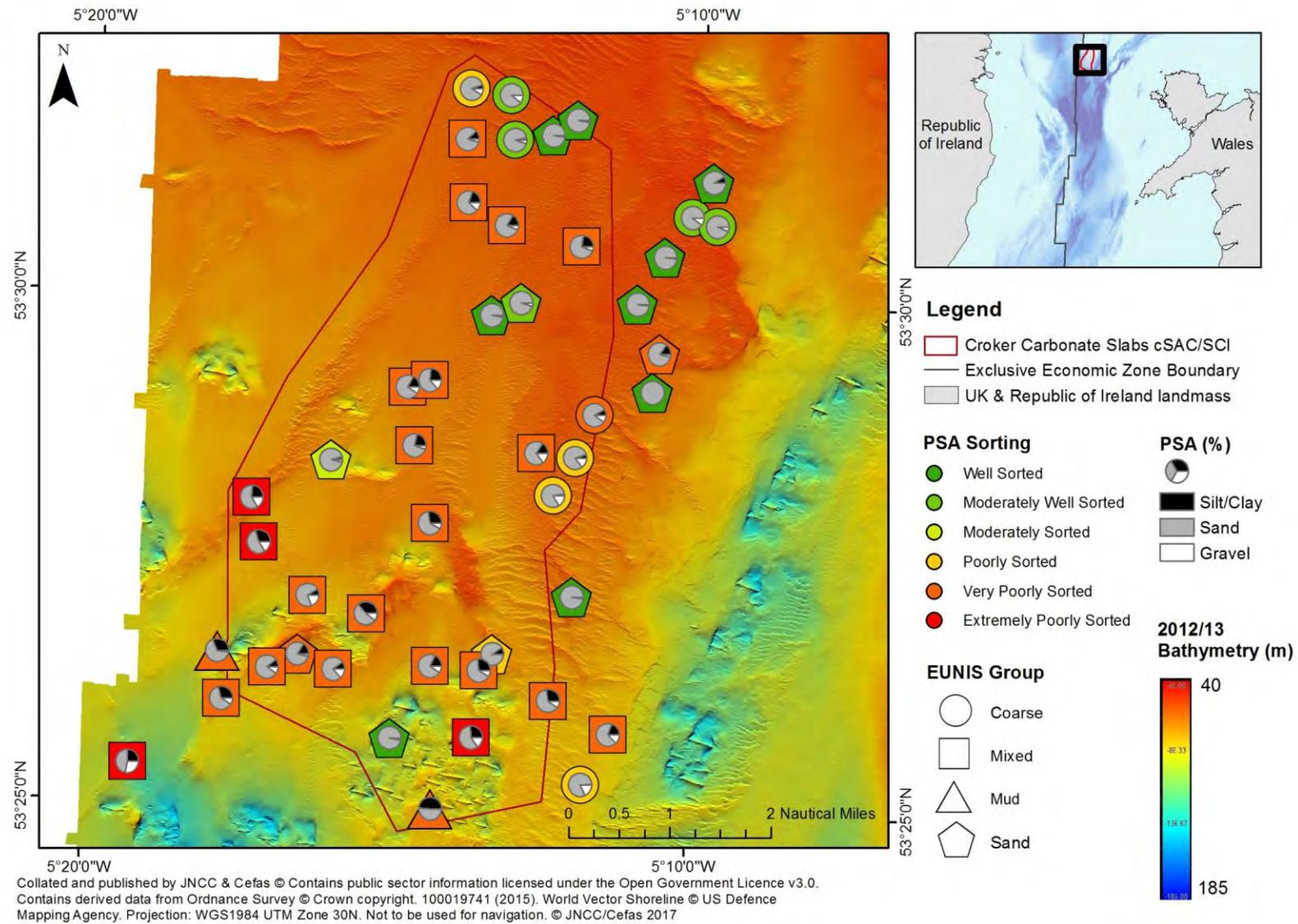
**Figure 4.** Grab stations with pie charts showing the results of particle size analysis, sediment sorting classifications and EUNIS level 3 habitat classifications, overlain onto 2012/13 MBES data.
