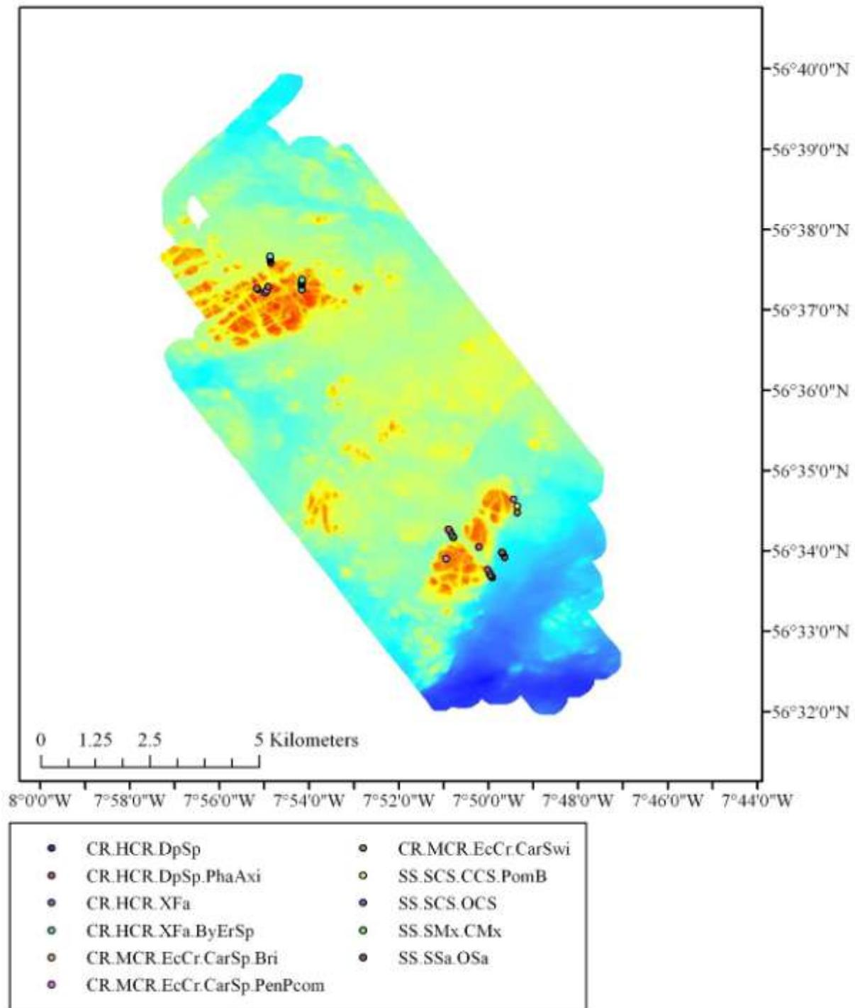
**Figure 2e.** Multibeam bathymetry for SW Barra Site with classed ground-truthing video tracks.
