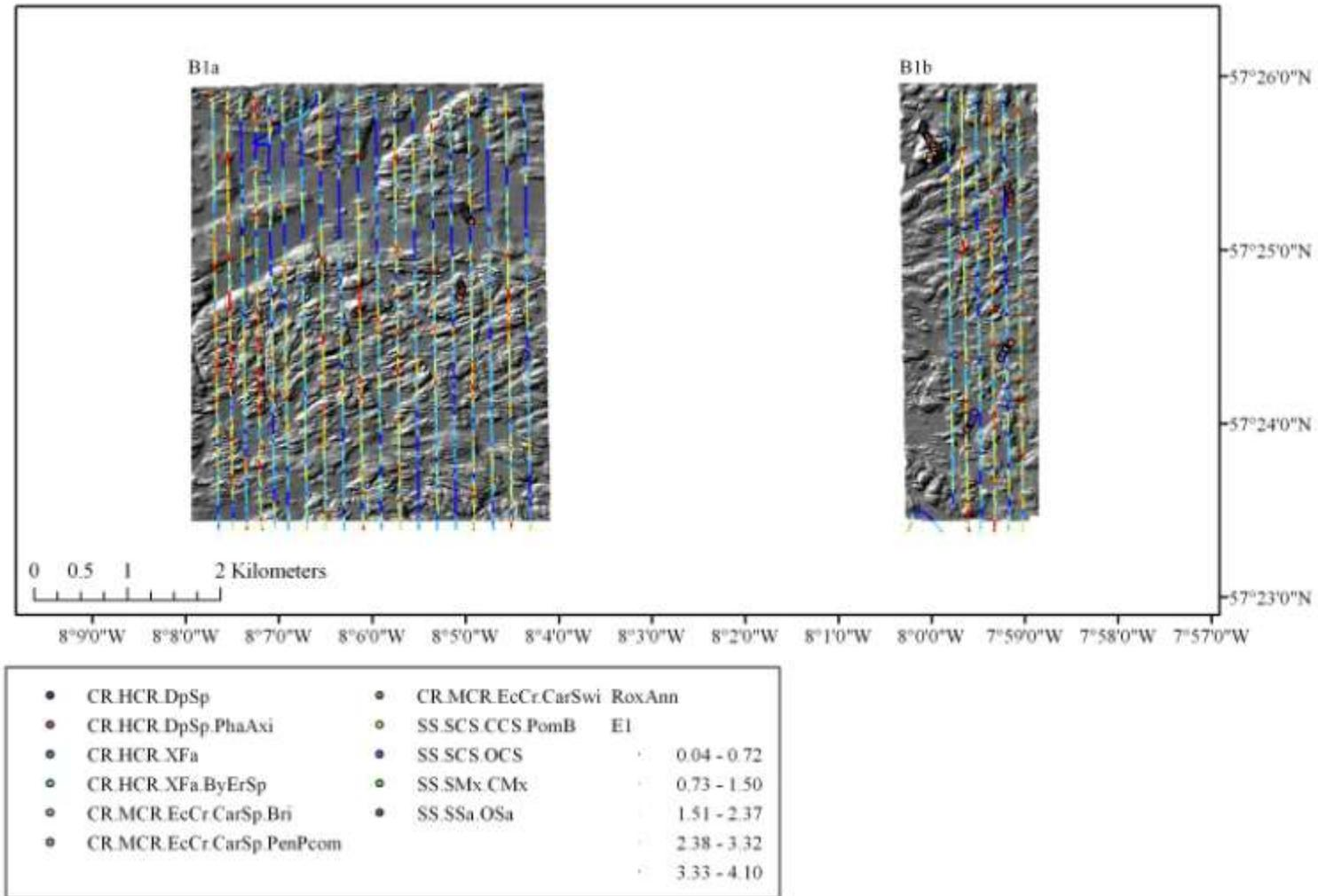
**Figure 3a.** Hillshaded multibeam bathymetry for Barra Site 1, with RoxAnn AGDS data overlaid (showing roughness- E1) and classed ground-truthing video tracks
