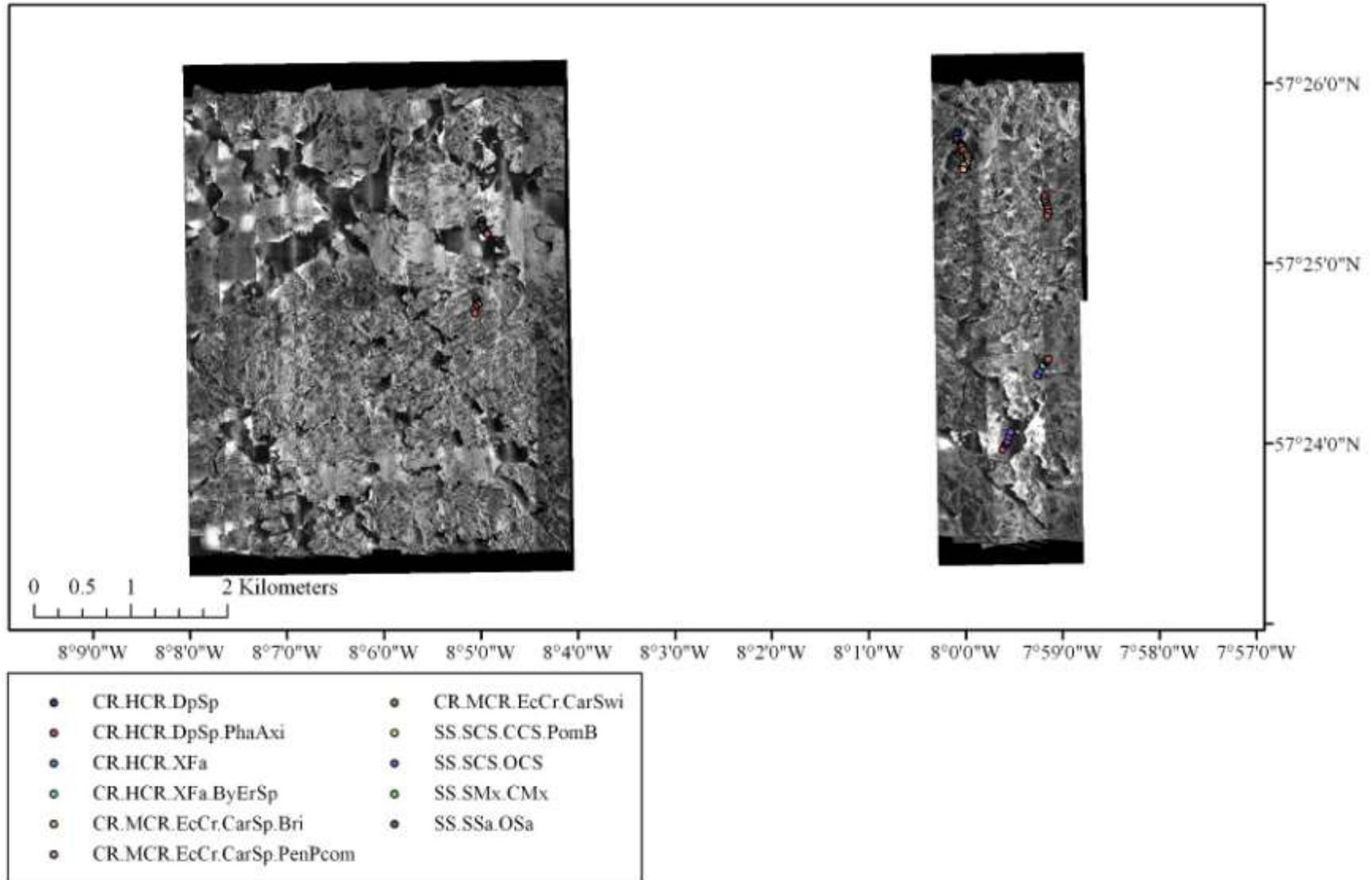
**Figure 6a.** Backscatter mosaics (processed using Caris SIPS software) for Barra Site 1, with classed ground-truthing video tracks overlaid.
