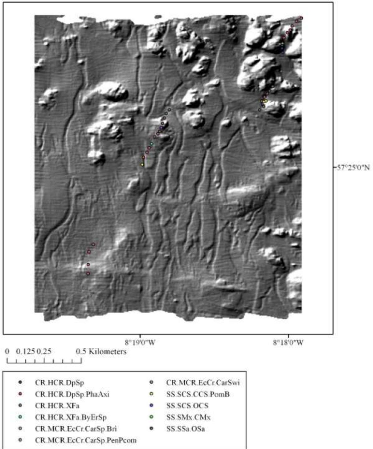
**Figure 3d.** Hillshaded multibeam bathymetry for Barra Site 5, and classed ground-truthing video tracks (no RoxAnn AGDS data available).
