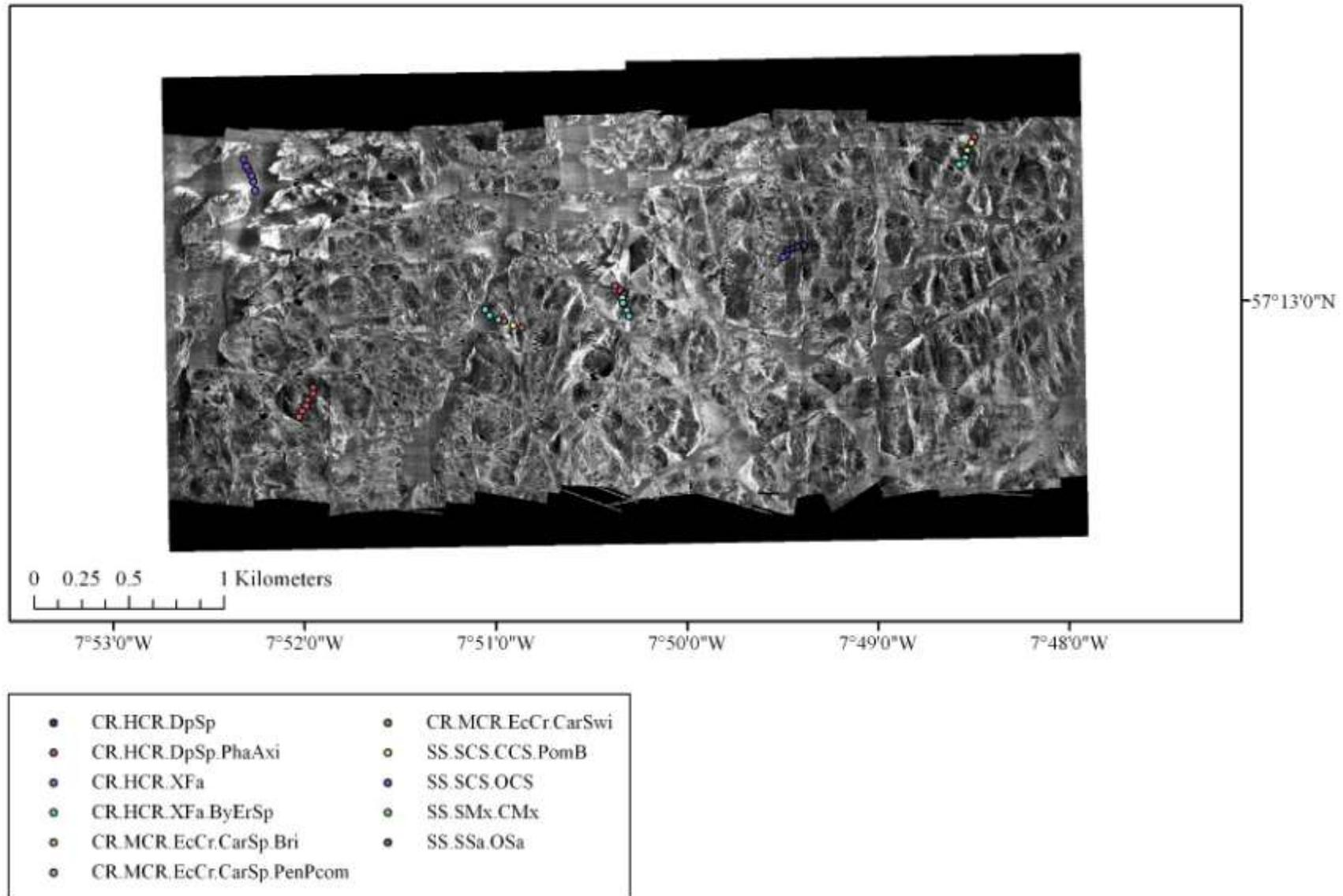
**Figure 6c.** Backscatter mosaics (processed using Caris SIPS software) for Barra Site 3, with classed ground-truthing video tracks overlaid.
