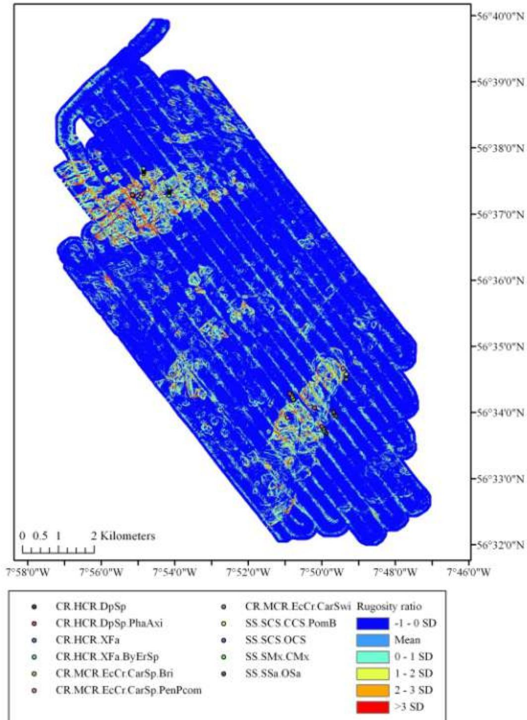
**Figure 5e.** Rugosity (classed into standard deviations) for SW Barra Site, with classed ground-truthing overlaid.
