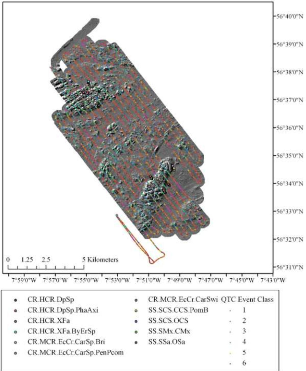
**Figure 3e.** Hillshaded multibeam bathymetry for SW Barra Site, with classed QTC-View AGDS data overlaid and classed ground-truthing video tracks.
