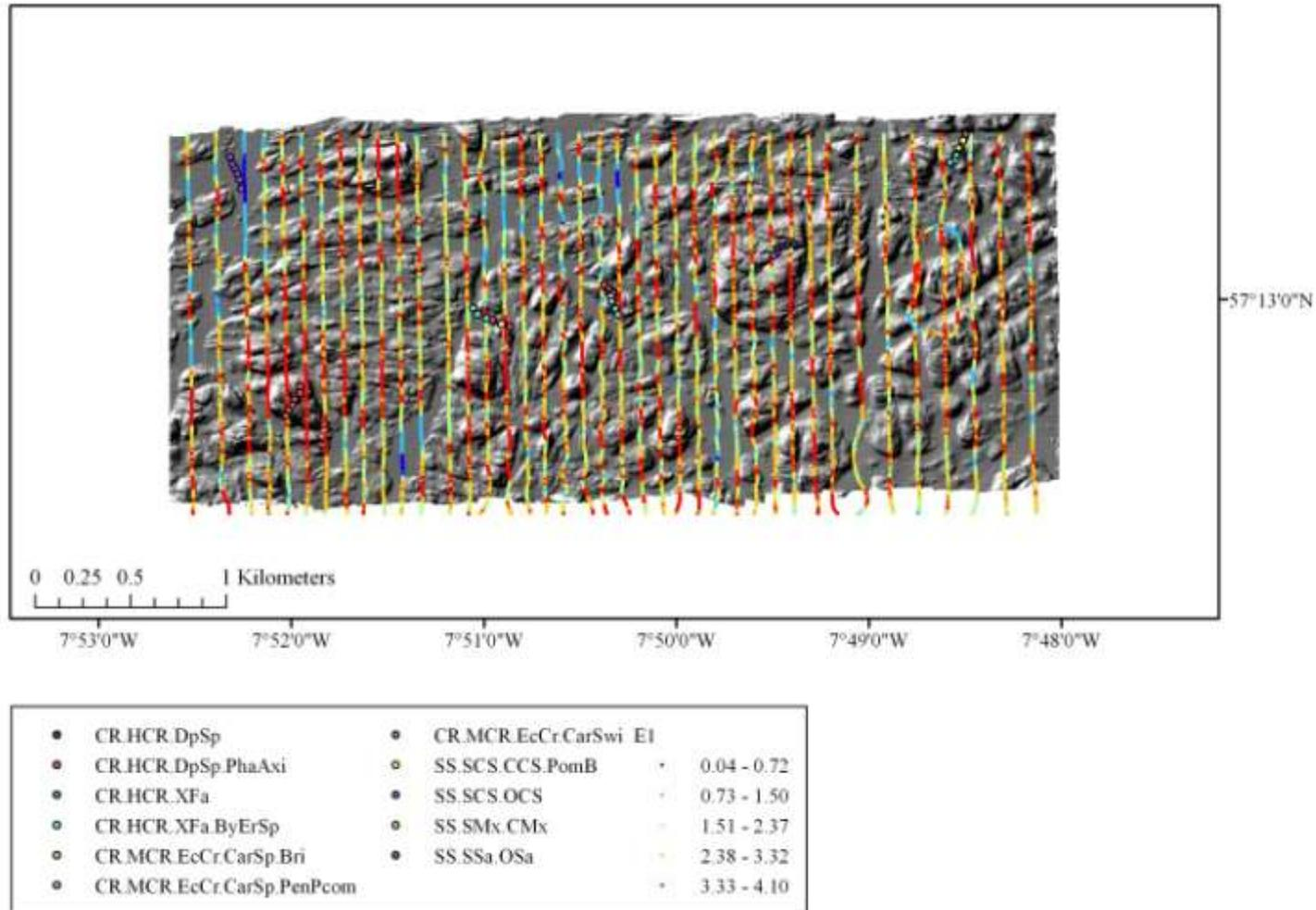
**Figure 3c.** Hillshaded multibeam bathymetry for Barra Site 3, with RoxAnn AGDS data overlaid (showing roughness- E1) and classed ground-truthing video tracks.
