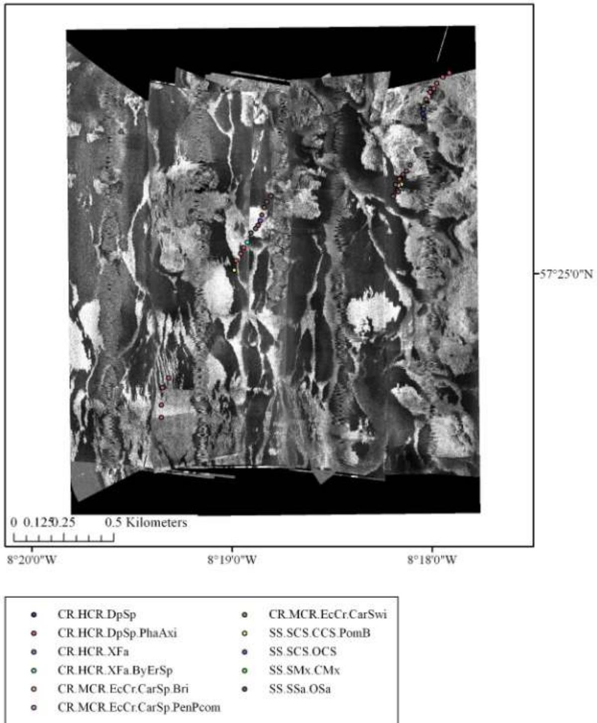
**Figure 6d.** Backscatter mosaics (processed using Caris SIPS software) for Barra Site 5, with classed ground-truthing video tracks overlaid
