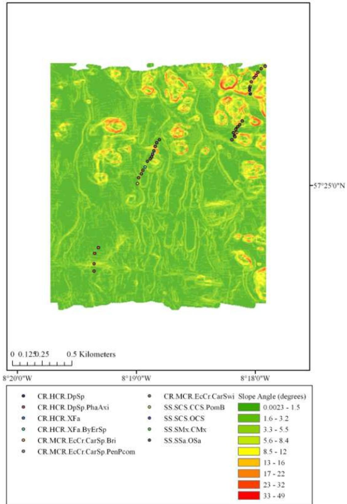
**Figure 4d.** Slope angle (in degrees) for Barra Site 5, with classed video ground-truthing overlaid.
