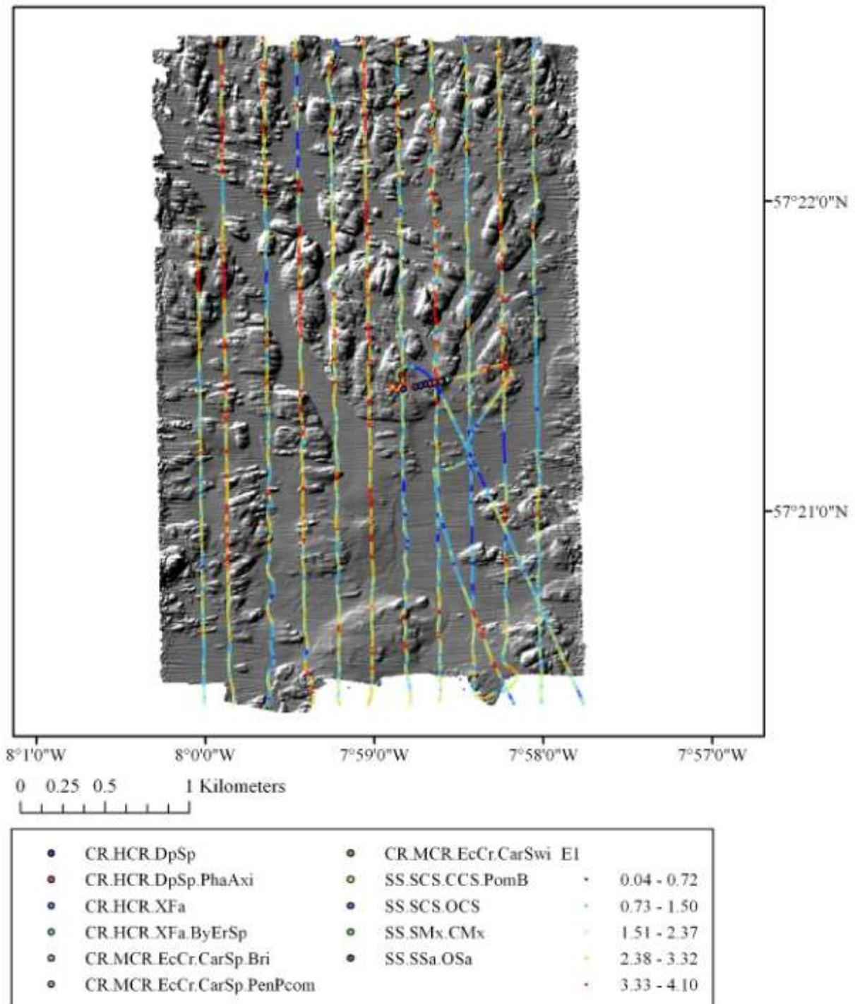
**Figure 3b.** Hillshaded multibeam bathymetry for Barra Site 2, with RoxAnn AGDS data overlaid (showing roughness- E1) and classed ground-truthing video tracks.
