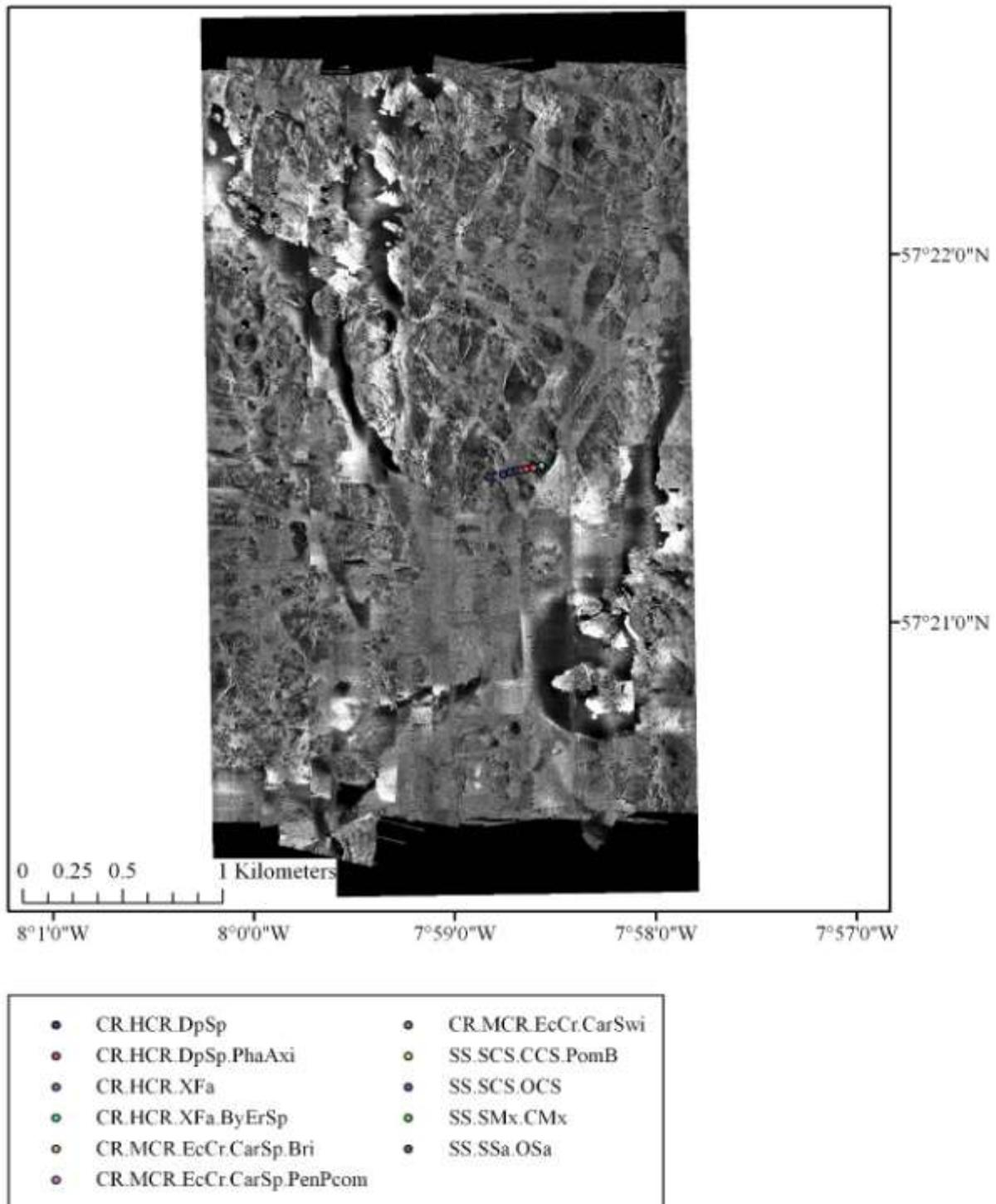
**Figure 6b.** Backscatter mosaics (processed using Caris SIPS software) for Barra Site 2, with classed ground-truthing video tracks overlaid.
