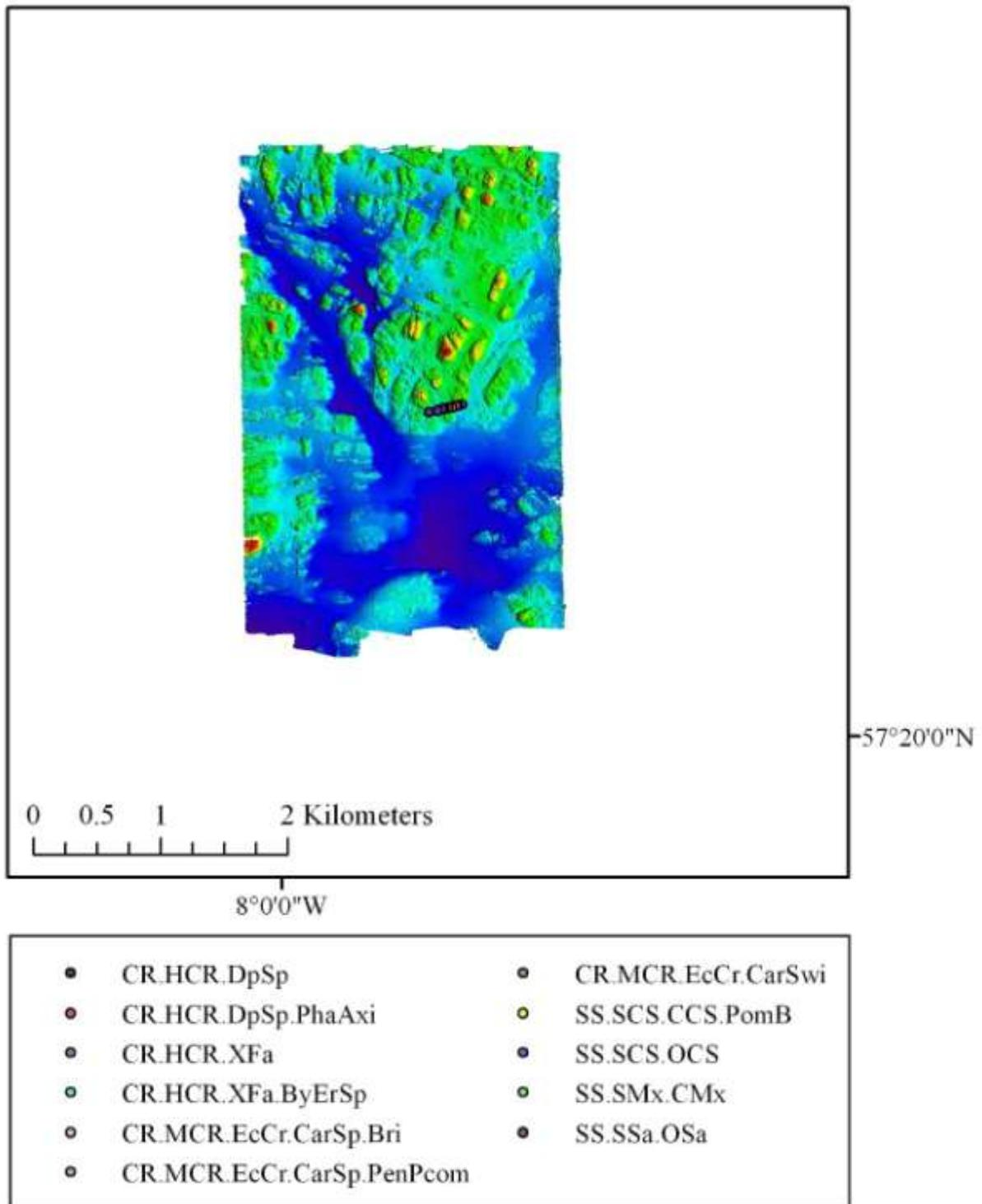
**Figure 2b.** Multibeam bathymetry for Barra Site 2 with classed ground-truthing video tracks overlaid.
