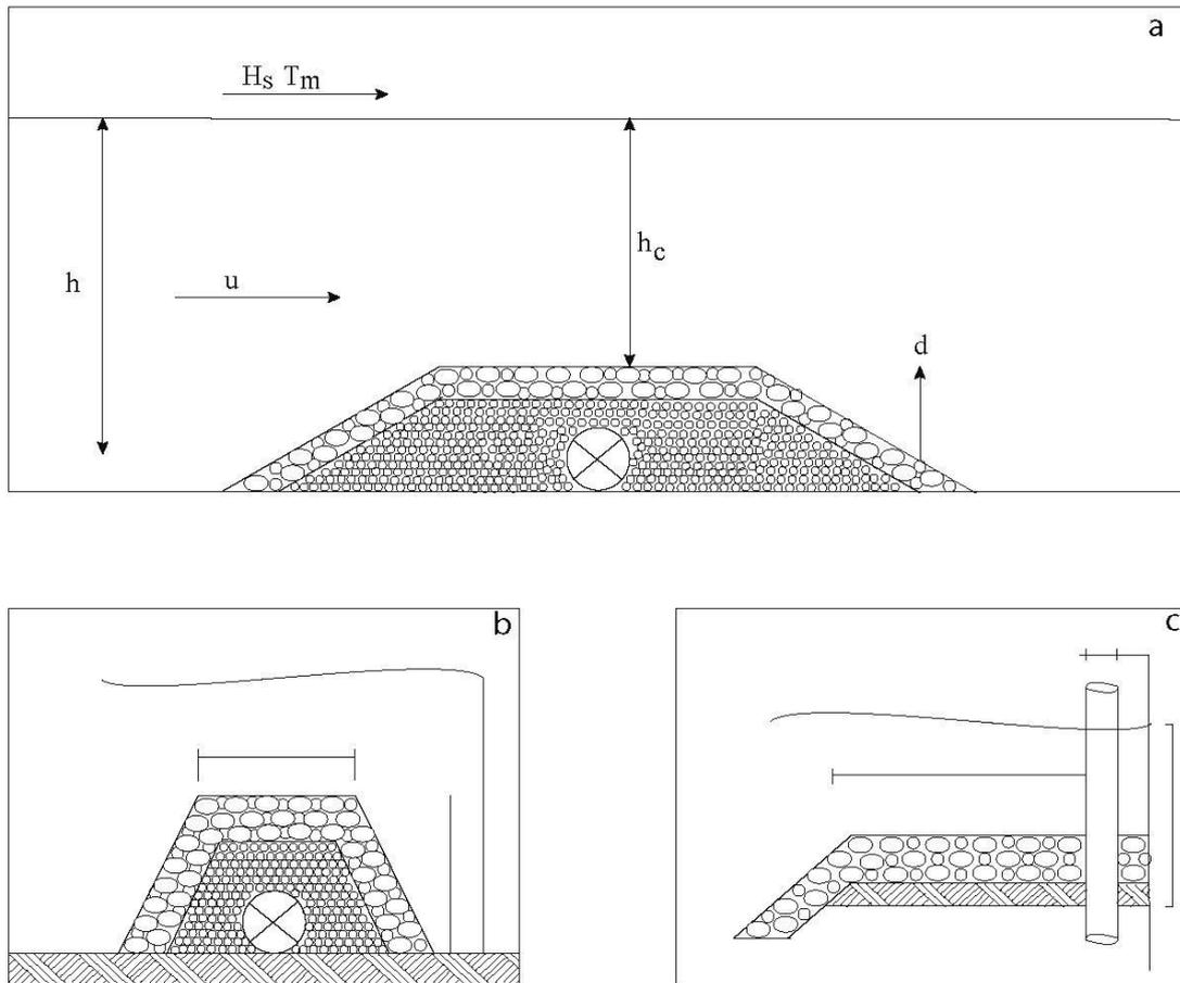
**Figure 9:** a) An overview of a typical rubble mound or rock protection method used for pipelines, including symbols for key parameters. b) An example of a pipeline protection rock berm. c) An example of a rubble mound used for the stabilisation of slender monopile-type foundations used in subsea infrastructure. Adapted from the CIRIA Rock Manual (2007).
