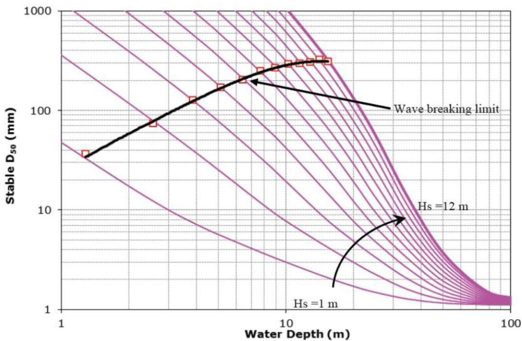
**Figure 10:** Stable  $D_{50}$  particle size required for  $U_c = 0.5 \text{ m.s}^{-1}$ ,  $T_s = 8 \text{ s}$  and  $H_s = 1 \text{ m} - 12 \text{ m}$  (from Thusyanthan *et al* 2013).
