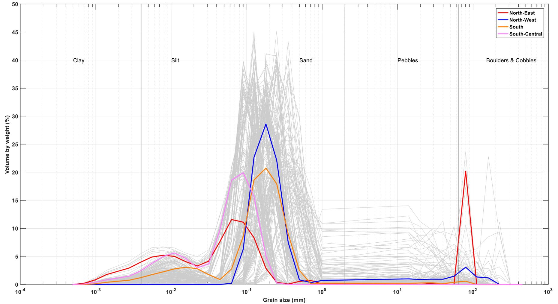
**Figure 7:** Particle size data obtained from Cefas for the NNSR cSAC/SCI. Four profiles have been highlighted for comparisons. The corresponding sites have been chosen according to geographic location within the site (see Figure 5 insert).
