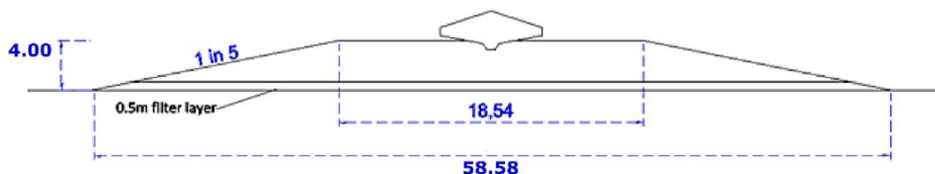
**Figure 11:** Cross-section of proposed rock placement under each jack-up leg at the Viking HD Platform. Source: ConocoPhillips Environmental Statement (2015) (Source: Global Maritime (2015)).
