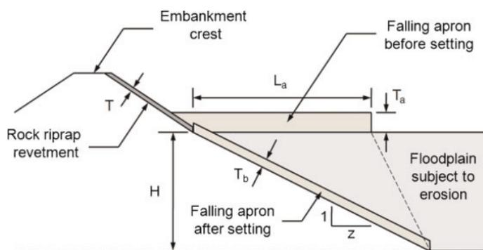
**Figure 8:** An example application of a 'falling apron' design used in rock dump for river bank stabilisation.
