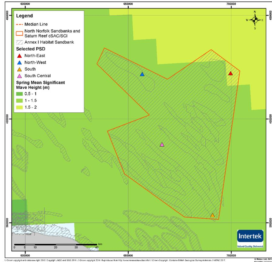
**Figure 4:** Typical wave height during mean spring tide (from ABPmer Tidal Atlas 2008).
