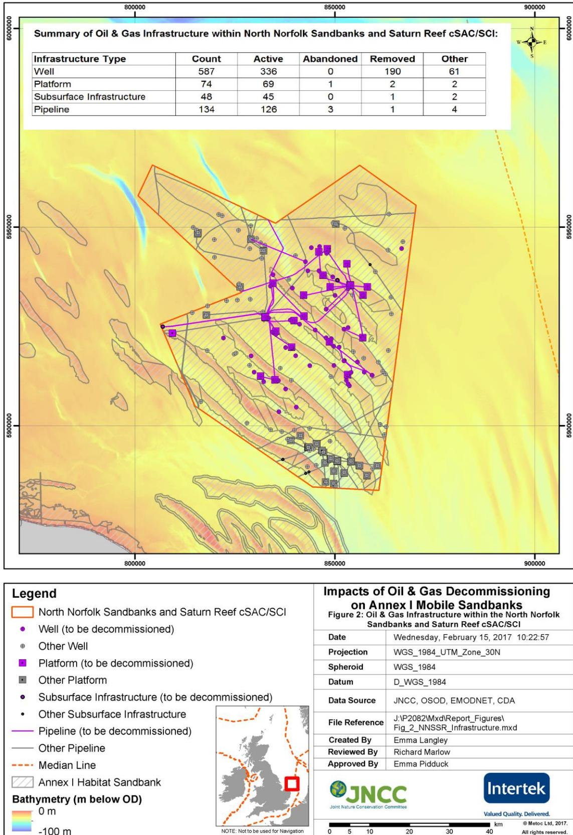
Figure 2: Oil and Gas infrastructure within the North Norfolk Sandbanks and Saturn Reef cSAC/SCI.
