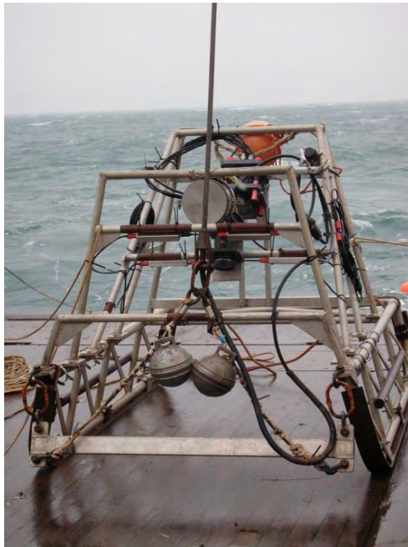
**Figure 6.** Image of the towed camera sledge comprising Kongsberg video and still image capture systems along with HD video acquisition system.
