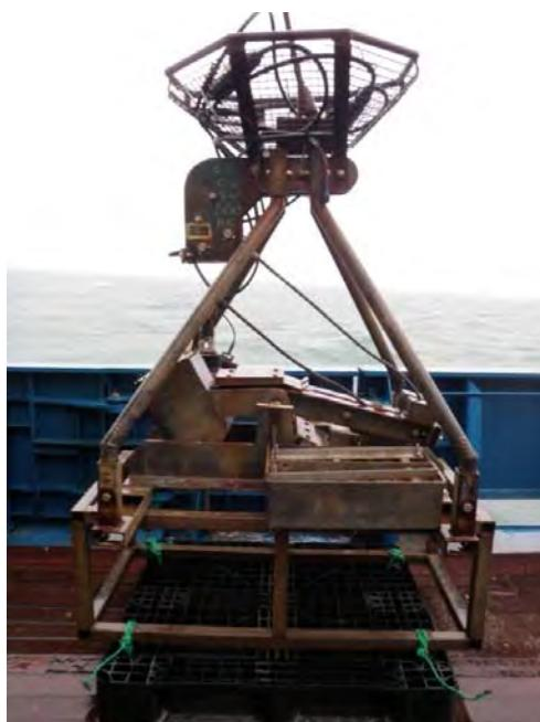
**Figure 4.** Image of the 0.1m<sup>2</sup> mini Hamon grab with video camera (collectively referred to as HamCam).
