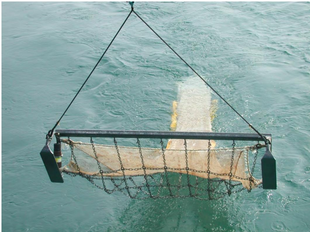
**Figure 7.** Image of the 2m scientific beam trawl utilised for epibenthic faunal sampling.
