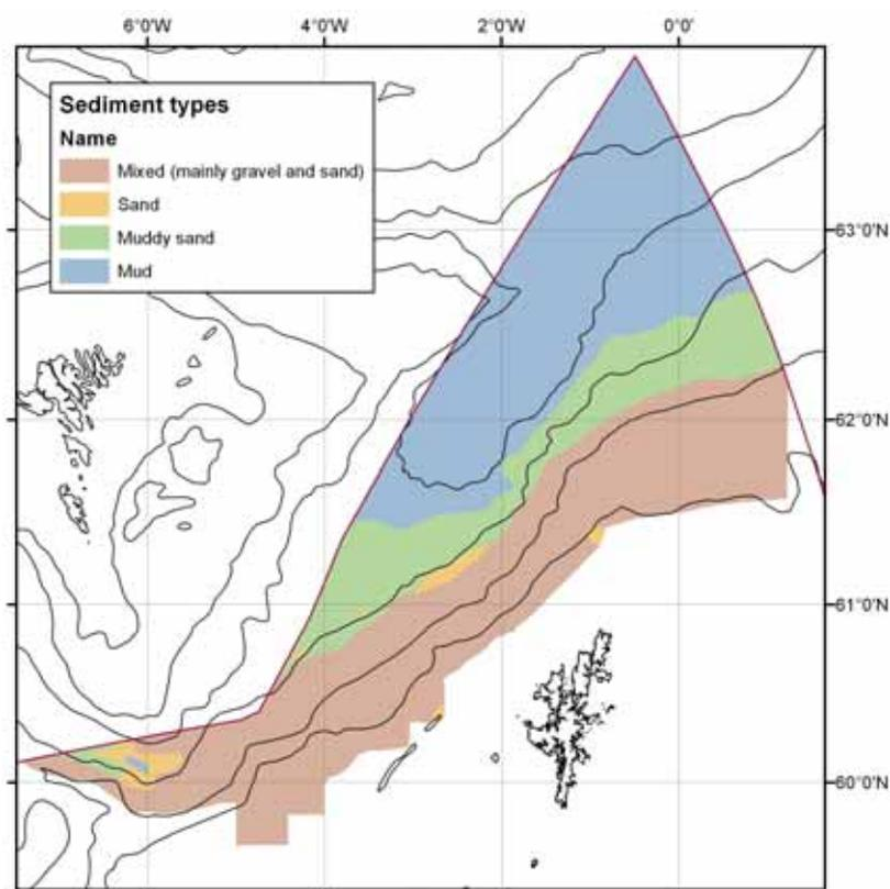
**Figure 5.** Generalised distribution of seafloor sediment types in the SEA4 area (adapted from Masson *et al* 2003). (The 200m contour and 500m-interval contours are shown, from GEBCO CE; IOC, IHO, BODC, 2003).
