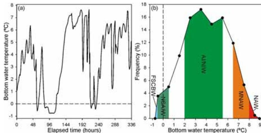
**Figure 4.** Temporal variability in West Shetland Slope bottom water temperatures. Data from a recording current meter moored 1.5m above the seabed in water depth of 550m, with temperature recorded at one-hour intervals for a period of 10-months. (a) Example data for a two-week period (3-16 February 1996). (b) Temperature frequency distribution for the 10-month period (15 September 1995-11 July 1996); water mass abbreviations, temperature bands, and colour coding follow those of Fig. 3.
